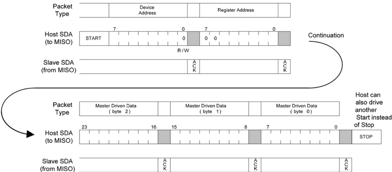
Figure 8. I2C 3 Byte Write Example
